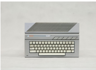
8 bit Atari 130 XE from the collection at the lab headed by the PI. One of the most important platforms for the demoscene and, at the same time, one with most hardware limitations, which the demosceners strive to overcome.
